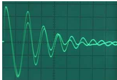
Figure 5. bad insulation between turns
